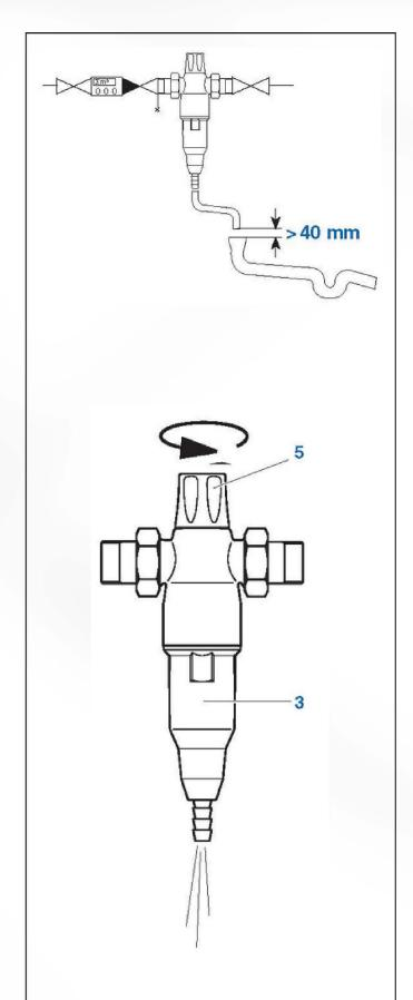
**Attention:** The installation site must be protected against frost and must ensure the protection of the filter against e.g. solvent vapours, fuel oil, lees, chemicals of any kind, UV radiation and heat sources above 40 °C.
