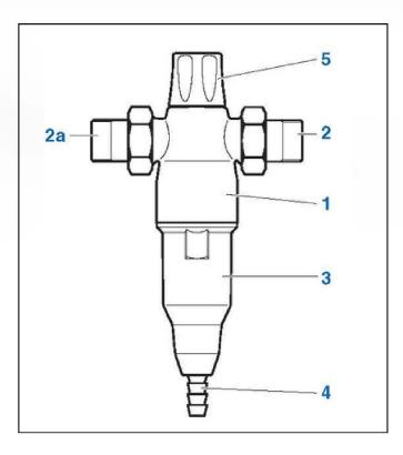
The particles on the filter cloth are removed by suction from the suction-ring backwashing system and then washed out.
