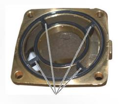
Align locating lugs and press gasket into groove
